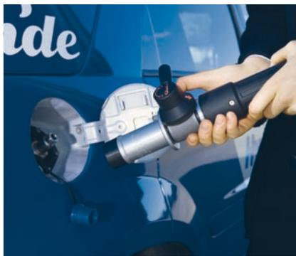
Refuelling coupling for filling compressed gaseous hydrogen
